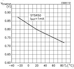
**Figure 21:** Start-up Voltage  $(V_{IN} - V_F)$  vs Temperature
