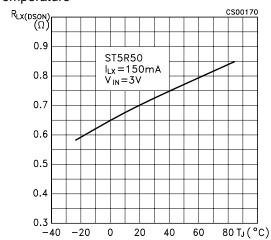
**Figure 27:** Internal Switch R<sub>DSON</sub> vs Temperature
