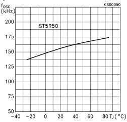
**Figure 15:** Maximum Oscillator Frequency vs Temperature
