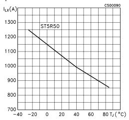
**Figure 19:** LX Switching Current Limit vs Temperature
