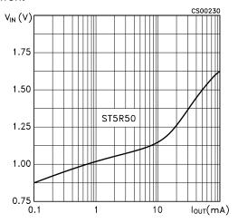
Figure 25: Minimum Input Voltage vs Output Current
