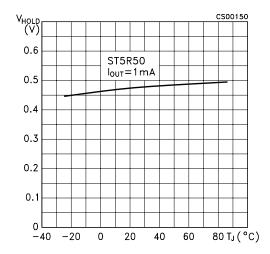
Figure 29: Hold-on Voltage vs Temperature
