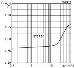
Figure 24: Minimum Input Voltage vs Output Current
