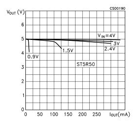
Figure 7: Output Voltage vs Output Current
