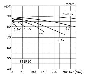
Figure 13: Efficiency vs Output Current
