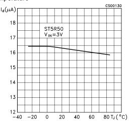
**Figure 31:** No Load Input Current vs Temperature
