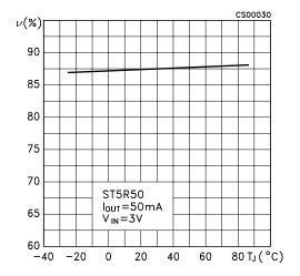
Figure 11: Efficiency vs Temperature
