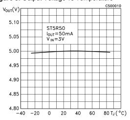
Figure 9: Output Voltage vs Temperature
