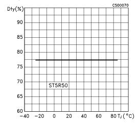
**Figure 17:** Oscillator Duty Cycle (@ MAX Freq.) vs Temperature
